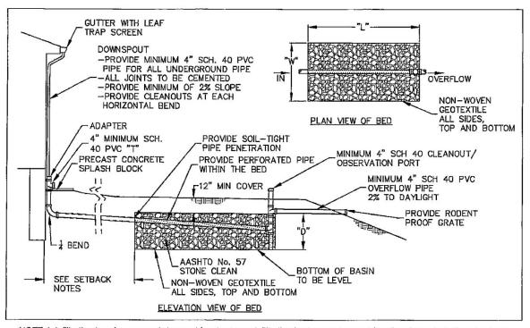
NOTE 1: Infiltration trenches may only be used for structures; infiltration basins may be used for all surfaces, including structures.
